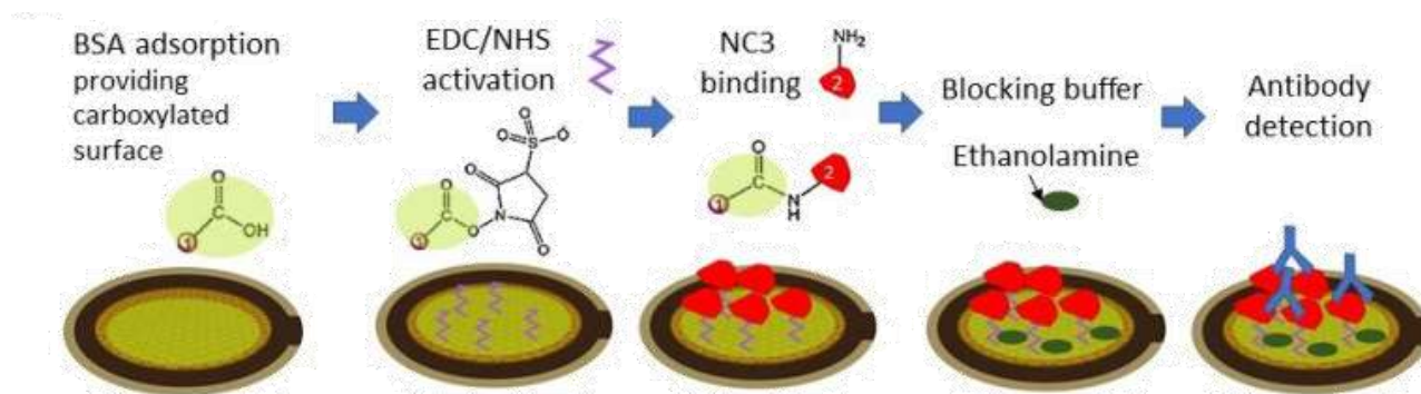
Figure 1: Schematic for functionalization of rGO surface to detect the antibodies starting with BSA adsorption, amine activation with EDC/NHS, immobilization of the receptor NC3 (in red) via amine covalent cross-link and blocking with ethanolamine.
