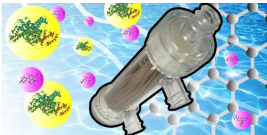
Figure 1: Core-shell hollow fiber PES-GO cartridge for synergic microfiltration and adsorption of microcontaminants from drinking water.
