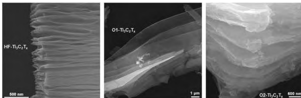
Figure 1: SEM images of pristine Ti 3 C 2 T x MXene sample (left) and different oxidation degrees of TiO 2 -Ti 3 C 2 T x heterojunction samples including lightly oxidized O1-Ti 3 C 2 T x (middle) and heavily oxidized O2-Ti 3 C 2 T x (right).
